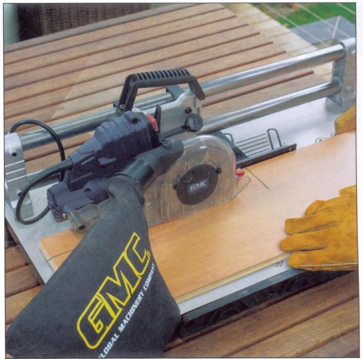
The width setting is adjusted by unscrewing a plastic knob and using the width markers cast into the base to set it.
