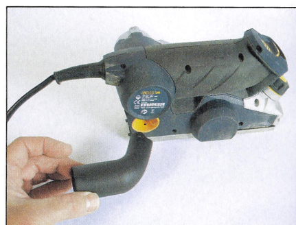
The dust extract adaptor fits into a port at the back
